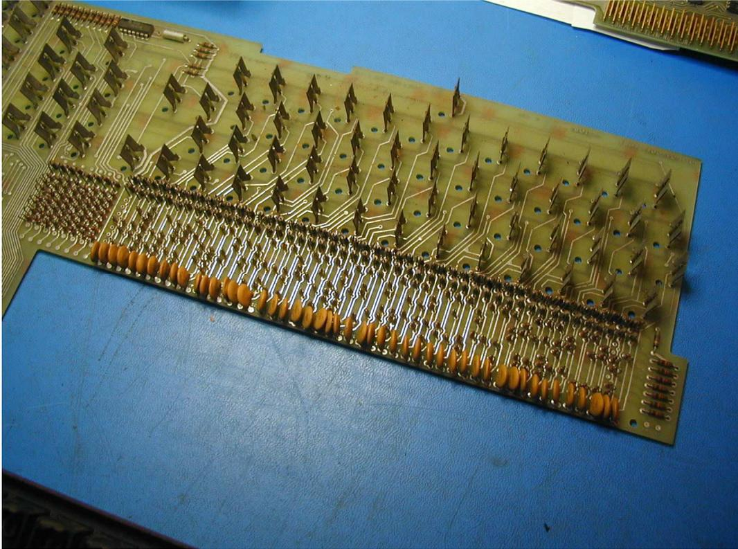
The reed switches can now be inspected and replaced if necessary. The top wire is welded to the metal bracket, but can be separated with a pair of sharp diagonal cutters. The new switch can be soldered instead.
