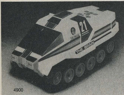
"Think Tank" from Vanity Fair is a keyboard programmed unit with 48 steps (right, left, straight, stop, etc.).
