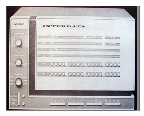
The 1968 Interdata Model 3 Control Computer could handle 16 and 32 bit instruction word lengths, had 1024 bytes of memory expandable to 65,536 bytes, 2 microseconds cycle time, and had 16-bit arithmetic and 16 general registers. It sold for about \$6,000.
