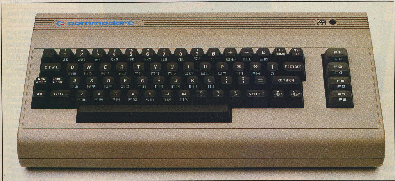
The Commodore-64 features expanded graphics capabilities, including three modes for displaying text (standard, multicolor and extended-color). The C-64 also features music-making capabilities, made possible by the MOS 6581 Sound Interface Device chip.
